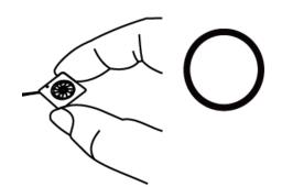
Don't pull fan with lead wires.
