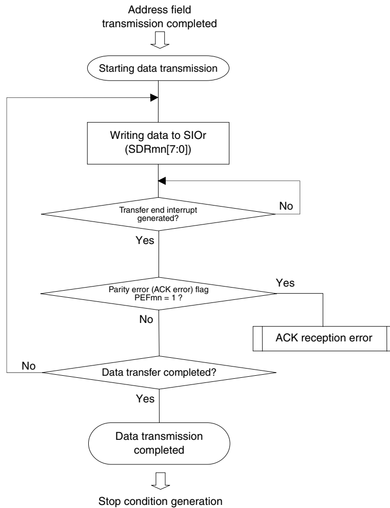
Figure 14-104. Flowchart of Data Transmission
