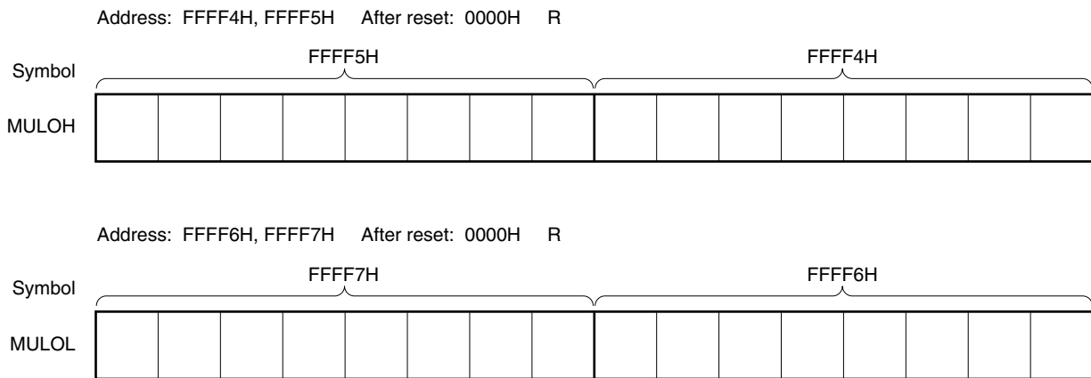
Figure 15-2. Format of 16-bit higher multiplication result storage register and 16-bit lower multiplication result storage register (MULOH, MULOL)
