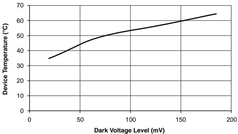
Figure 9. KLI-8023 Typical Dark Voltage Level vs. Temperature
