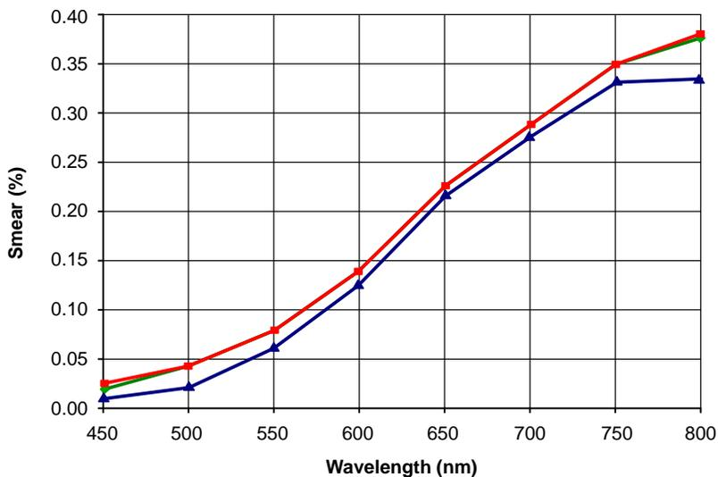
Figure 7. KLI-8023 Smear – LDR Operation/1 MHz/35°C
