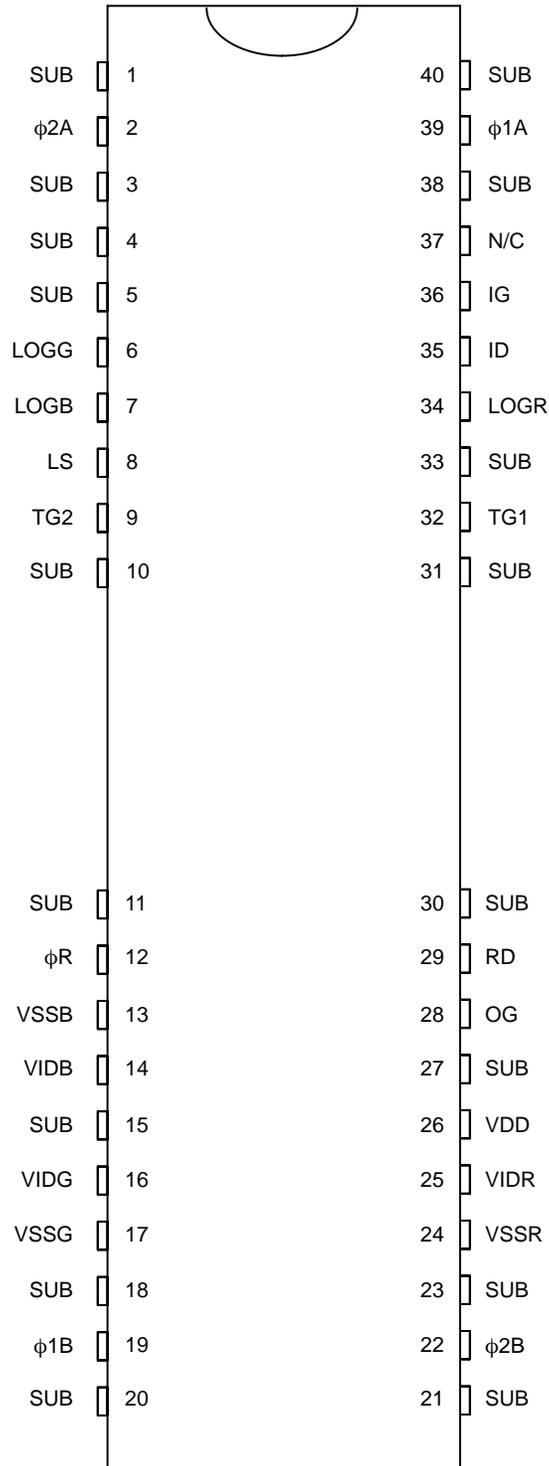
Figure 3. KLI-8023 Pinout
