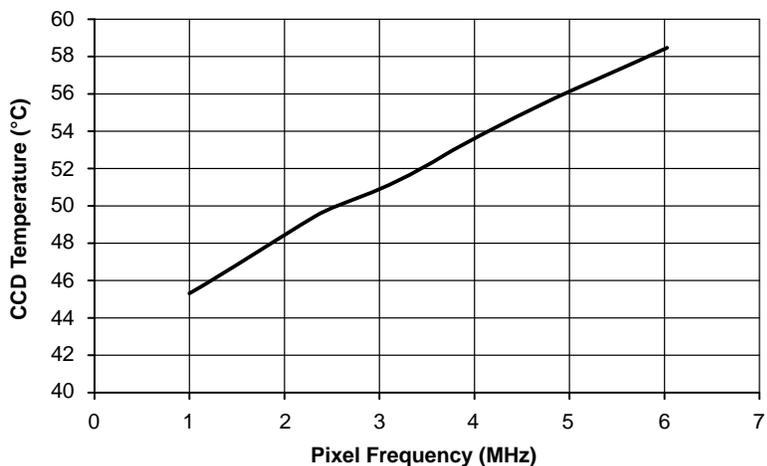
Figure 10. KLI-8023 Typical CCD Temperature vs. Operating Frequency
