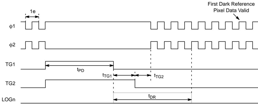
Figure 17. Photodiode-to-CCD Transfer
