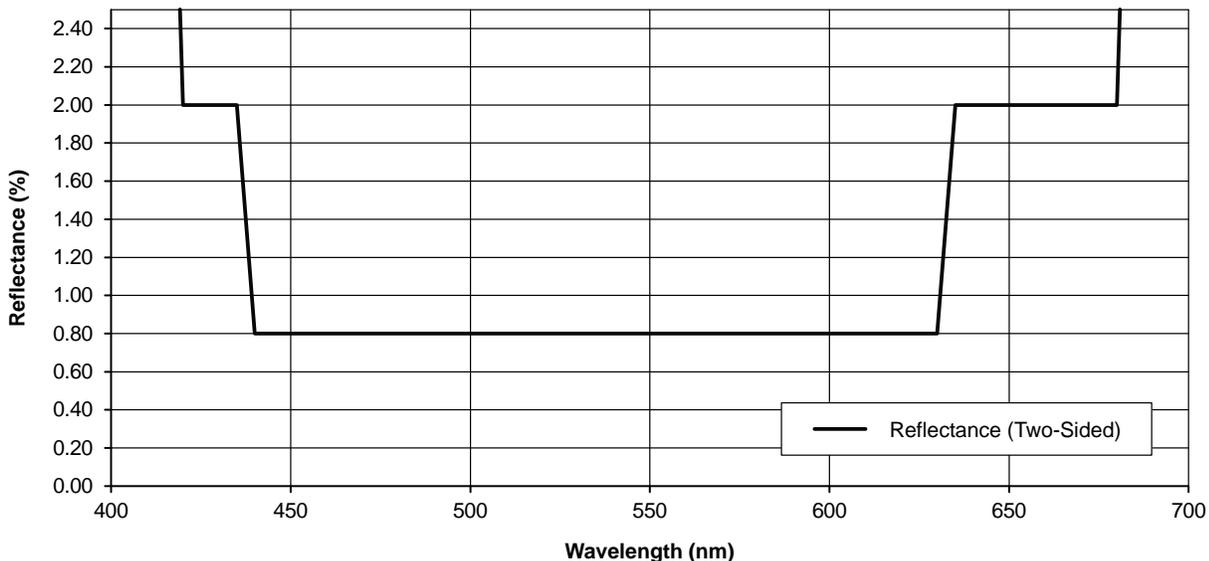
Figure 21. Two-Sided Multilayer Anti-Reflective Cover Glass Specification (MAR)
