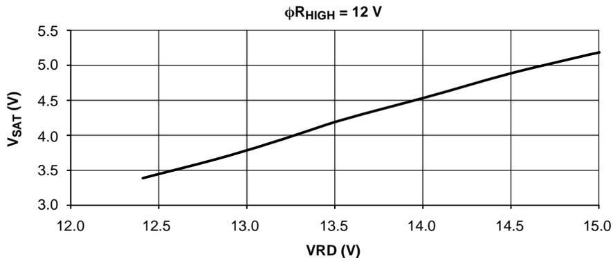
Figure 8. KLI-8023 Typical Saturation Voltage vs. VRD
