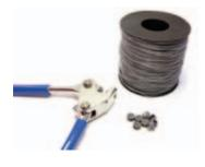
Pliers, steel wire and lead seals used to seal the auxiliary release device (head 96D).
