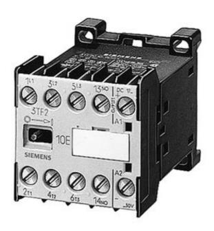
CONTACTOR SIZE 00 3-POLE AC-3 4KW/380V, AUX. SWITCH 11 (1NO+1NC), WIDTH 90 MM PIN, JACK CONNECTION 6.3 MM, DC ACTUATION 24 V DC
