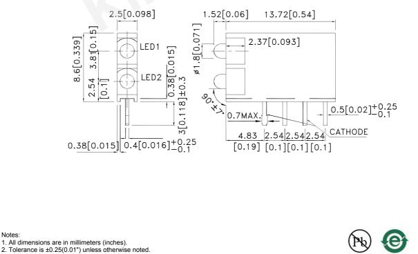
Lead spacing is measured where the leads emerge from the package.
