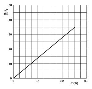
Hot-spot temperature rise ( $\Delta \emph{T})$  as a function of dissipated power
