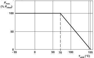
Maximum dissipation ( $P_{\text{max}}$ ) in percentage of rated power as a function of the ambient temperature ( $T_{\text{amb}}$ )
