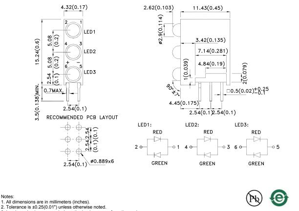
Lead spacing is measured where the leads emerge from the package.
