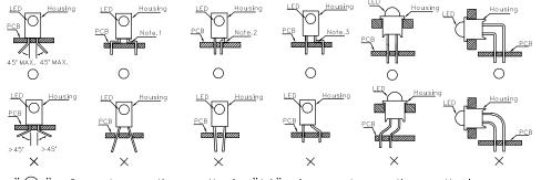
"○" Correct mounting method "X" Incorrect mounting method Note 1-3: Do not route PCB trace in the contact area between the leadframe and the PCB to prevent short-circuits.
