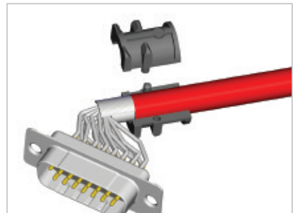
Attach the strain relief around the cable
