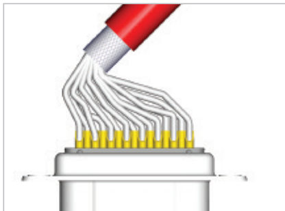
Strip cable 18mm and shape cable to two pigtailed
