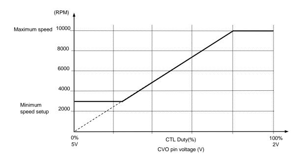
(1) Obtain the ratio of the minimum speed required to the maximum speed.
