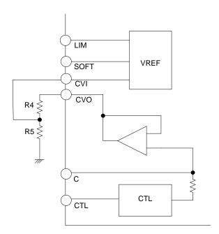
(2) Movement along the Y-axis (resistance divided between CVO and V<sub>CC</sub>)
