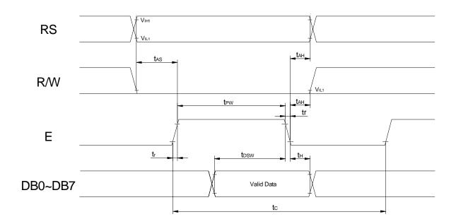
10-2-2 Read mode (Reading data from module to MPU)
