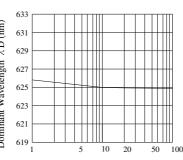
Forward Current IFP (mA) Ambient Temperature vs. Dominant Wavelength
