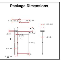
the LED chip was in reverse polarity, which is different from normal LED, please check the polarity of the LED before production. And please be noted that BIGGER side of the LED is "+ve""
