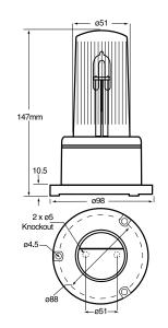
The X125 Din Base Series utilises a discharge capacitor and converter circuit to ignite xenon gas inside a tube, resulting in a brilliant flash of light. Xenon gas ignites virtually instantaneously so maximum brightness is obtained
