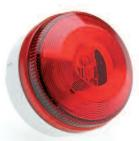
The X195 Series utilises a discharge capacitor and converter circuit to ignite xenon gas inside a tube, resulting in a brilliant flash of light. Xenon gas ignites virtually instantaneously so maximum brightness is obtained immediately. Xenons
