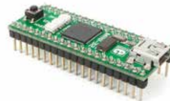
MIKROE-763 MINI-32 contains PIC32MX534F064H
