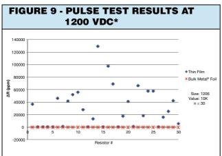
\* Note: Average of 30 units yielded deviation of 30,723 ppm of the Thin Film vs. -14 ppm for the Bulk Metal® Foil
