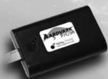
Aardvark I2C/SPI Host Adapter
