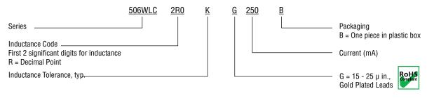
The above part number refers to a 506WLC Series 2.0 µH inductor, K tolerance (±10%, typ.), with Gold Plated Leads (G), 250 mA, one piece in plastic box.
