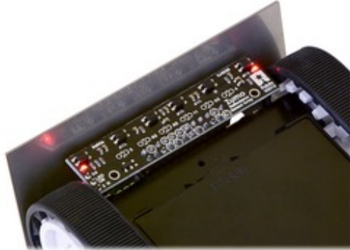
Zumo reflectance sensor array on a Zumo robot, bottom view.
