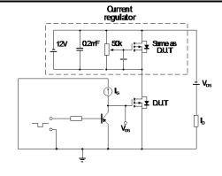
Gate charge test circuit
