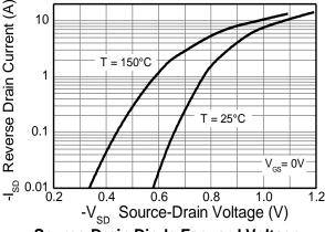
**Source-Drain Diode Forward Voltage**
