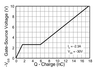
**Gate-Source Voltage v Gate Charge**
