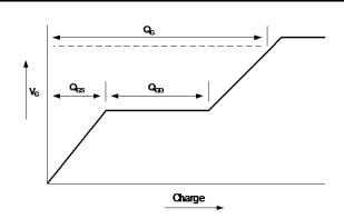
Basic gate charge waveform
