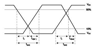
Switching time waveforms
