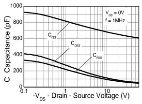
**Capacitance v Drain-Source Voltage**
