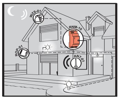
4-channel radio modular transmitter RNM-10 can control any EXTA FREE receiver. In this application RNM-10 is released by a signal from WZS-01 twilight switch, it sends a control signal to ROP-01 receiver, which switches on external lighting.
