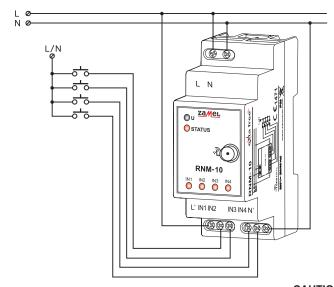
**CAUTION:** power supply must be connected to L' i N' terminals
