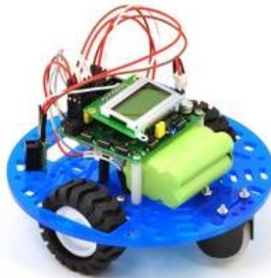
Pololu 5" round robot chassis RRC04A includes two spacers.
