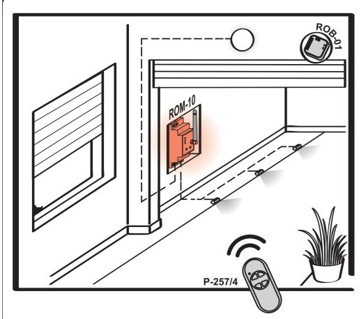
Radio modular receiver ROM-10 operates as a receiver of P-257/4 4-channel remote control (control of lighting operation in front of and inside the garage). Additionally P-257/4 remote control can control operation of ROB-01/12-24V radio gate controller.
