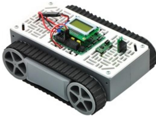
A narrow RP5/Rover 5 expansion plate with an Orangutan SV-328 and a Sharp digital distance sensor.
