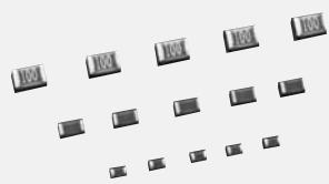
Resistors with high power in small size are realized as 1/3W for 2.0×1.25mm(0805) size, 1/5W for 1.6×0.8mm(0603) size and 1/6W for 1.0×0.5mm(0402) size.
