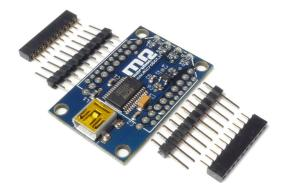
The *XBee to USB Adapter* is an usefull tool that allows to connect Personal Computers or a microcontroller in wireless networks using the famous XBee wireless modules. Connection is done via USB port and when you plug the board into the USB port, the PC system will recognize it as a serial VirtualCOM Port (VCP) which will realize the communication with the XBee module.
