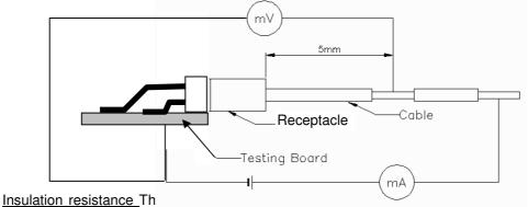
Insulation resistance Th  $\alpha$  an 1000 M $\Omega$  when measured in accordance with MIL-STD-202, Method 302. The following details shall apply
