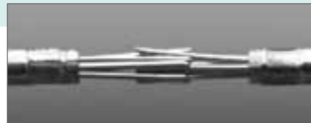
Bristle Brush Contacts - Multiple Strands of Wire are Bundled together to form a "Brush-like" Contact
