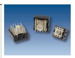
The RADSOK® PowerBlok™'s compact footprint 1/2" x 1/2" can supply up to 70A to backplane power connections. Current is distributed over 16 compliant pins. The PowerBlok™ is available for top or bottom entry and offered with a touchproof cover.
