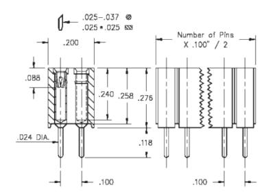
**Description:** Interconnect Socket Standard Solder Tail Socket Accepts .025" - .037" (0,635 - 0,94 mm)dia leads Double Row Through Hole **Plating Code:**
