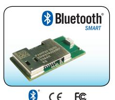
The **PAN1720 Series** is an ideal choice for applications where battery life is a critical application requirement, using only 500 nA in sleep mode. Short transition times between operating modes – 3uS Wake-Up – and power efficient hardware further reduce current consumption.
