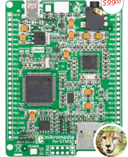
mikromedia for STM32 (features STM32F207VGT6 or STM32F407VGT6)
