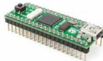
MIKROE-763 MINI-32 contains PIC32MX534F064H
