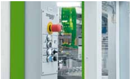
For Emergency Stop functionality the DA1 has the STO function built in.
