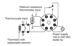
On the E52-□□1D, the lead wires are thermocouple element wires, making them difficult to solder because solder will not stick to them easily. Remove the crimp terminal and polish the ends before attempting to solder them.
