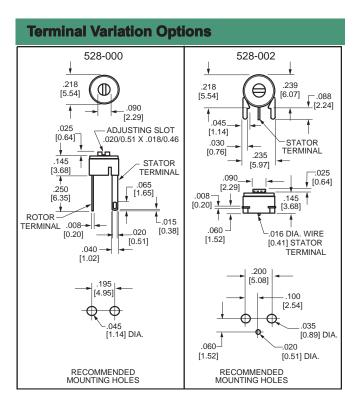
For dimensions  $\geq$  .126"/3.20mm, tolerance is  $\pm$ .015/0.38 For dimensions  $\leq$  .125"/3.18mm, tolerance is  $\pm$ .005/0.13
