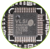
Figure 8-1: On-board VS1053 MP3 codec
