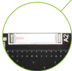
Figure 16-1: 2.4GHz ceramic chip antenna
