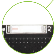
Figure 16-1: 2.4GHz ceramic chip antenna
