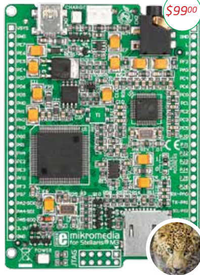
mikromedia for Stellaris M3 (features LM3S9B95)
