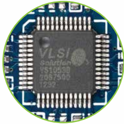
Figure 8-1: On-board VS1053 MP3 codec
