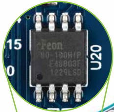
Figure 12-1: Flash memory module
