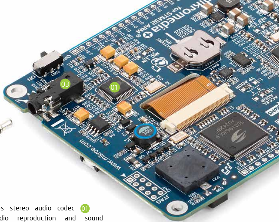
Figure 8-1: On-board VS1053 MP3 codec
