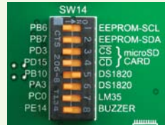
Figure 20-3: Enabled SW14.5 DIP switch
