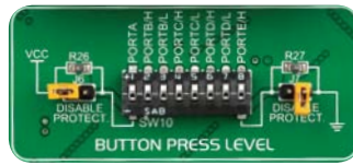
Figure 6-5: Button press level DIP switch (tri-state)
