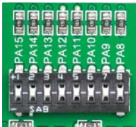
Figure 6-2: Tri-state DIP switch on PORTA/H
