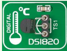
Figure 20-2: DS1820 correctly placed in socket
