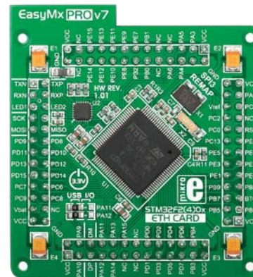
Standard 100-pin HP ETH MCU card with STM32F407VGT6
