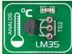
Figure 21-2: LM35 correctly placed in socket
