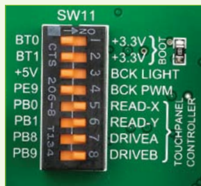
Figure 17-2: Turn on switches SW11.5 , SW11.6 , SW11.7 and SW11.8 to enable Touch panel controller
