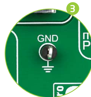
Figure 26-1: Three oscilloscope GND pins are conveniently positioned so different parts of the board can be reached with an oscilloscope probe
