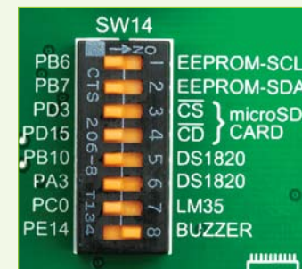
Figure 25-2: push SW14.8 to ON position to connect Piezo buzzer to PE14
