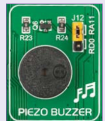
Figure 19-2: Use jumper J12 to connect Piezo buzzer on R20 or RA11 pin
