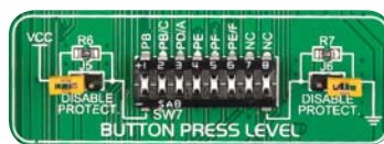
Figure 10-6: Button press level DIP switch (tri-state)
