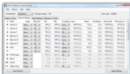
The Channel Settings tab in the Maestro Control Center.
