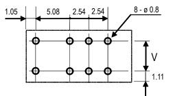
EE2 Series (top view) Non-latch type and single coil latch type
