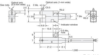
$\ast$  Vinyl-insulated round cable of 3.5 dia., 3 cores, (0.14 mm^2 with 1.0-dia. insulator); Standard length: 1 m
