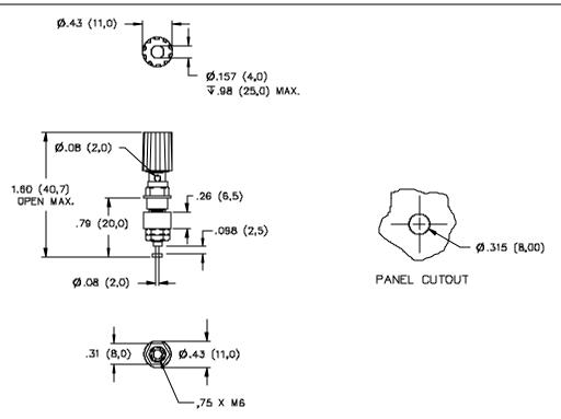
Recommended Maximuml Panel Thickness: .12" (3,0mm)
