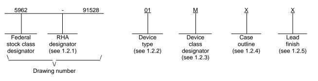
1.2.1 <u>RHA designator</u>. Device classes Q and V RHA marked devices meet the MIL-PRF-38535 specified RHA levels and are marked with the appropriate RHA designator. Device class M RHA marked devices meet the MIL-PRF-38535, appendix A specified RHA levels and are marked with the appropriate RHA designator. A dash (-) indicates a non-RHA device.
