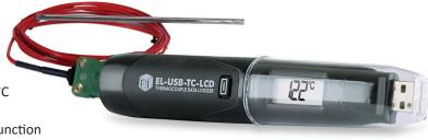
This standalone data logger measures and stores more than 32,000 temperature readings from a J, K or T-type thermocouple at a resolution of  $0.5^{\circ}$ C (1°F). It comes supplied with a K-type thermocouple capable of measuring from 0 to 200°C (32 to 392°F).
