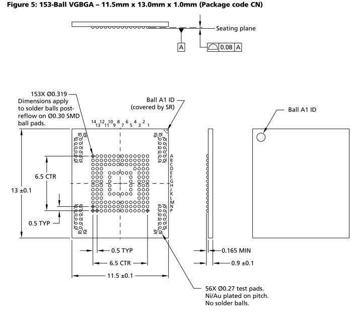
Note: 1. Dimensions are in millimeters.
