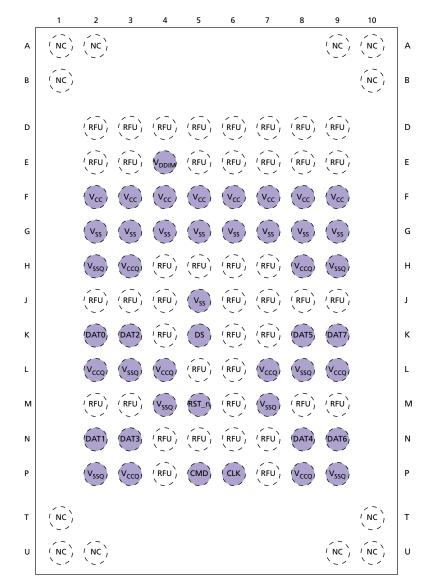
Notes: 1. Connect a  $1\mu$ F decoupling capacitor from V<sub>DDIM</sub> to ground.
