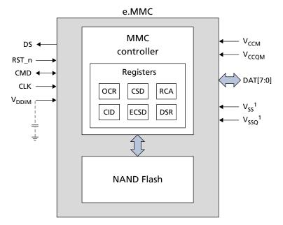
Note: 1. V<sub>ss</sub> and V<sub>ssQ</sub> are internally connected.
