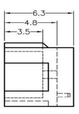
To weld  $\phi 5$  LED on board with 90 degrees, and same height, but avoid pins broken. Be used in combination.
